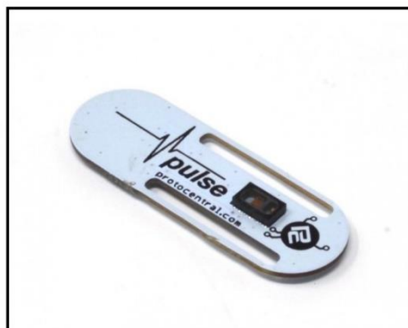
Figura 1: Pulse+ Pulse-OX & Heart Rate Sensor baseado no Max30102
